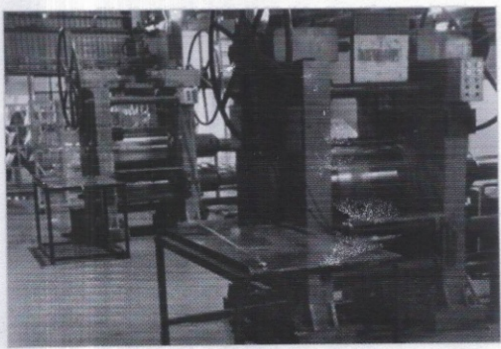
4 Hi mill machine using for rolling the material to make reducing the thickness
