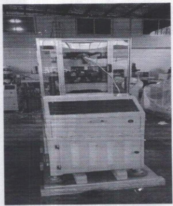
Fin Forming machine used for making corrugated fins for transformer
