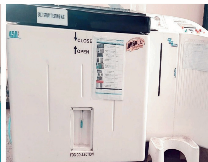
Salt Spray Test
